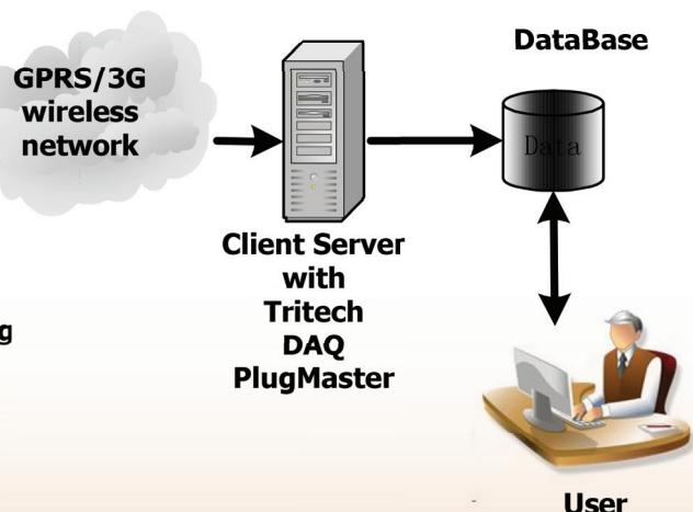
Customer can access the data any time in any of the electronic device, by connecting to the SQL database directly via standard SQL query. Data viewable includes real-time value of any parameter, system operating status like system voltage, data logger's health and etc. This great feature enables the customer to have in-time and in-depth information about the far-away monitoring station, without having the hassle to go down and download the data manually.
